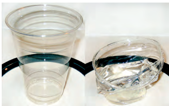
Fig. 2. The effect of hot water on PLA cups – T_g is the glass transition temperature, above which the polymer becomes plastic and returns to its original size. https://publi.cz/books/180/06.html [09.12.2015]
